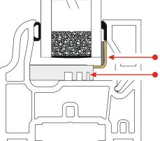
SECURI-CLIP Use SC147 for 24mm units Use SB000 Base Plate with GT016 White Packer
