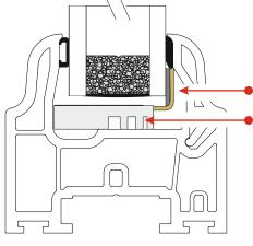
SECURI-CLIP Use SC147 for 24mm units Use SB000 Base Plate with GT016 White Packer
